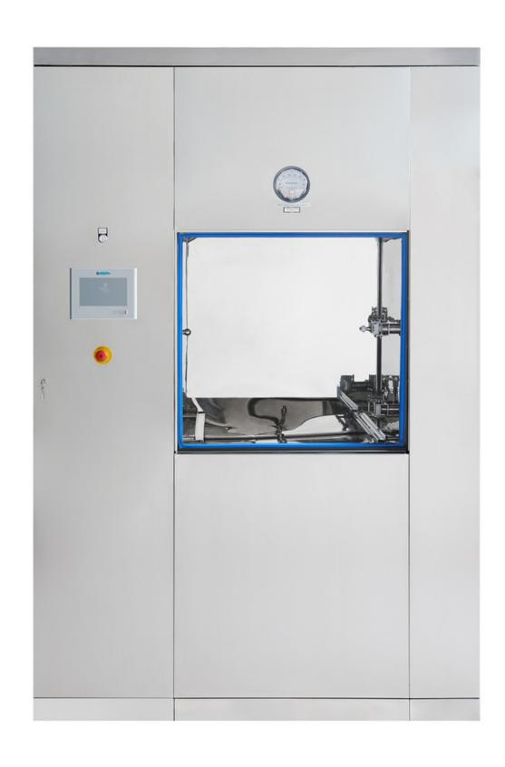
**AQUA** is particularly designed for process cleaning-disinfection and complete drying of materials used in the QC laboratories such as glassware, metal parts, plastic and rubber components.
